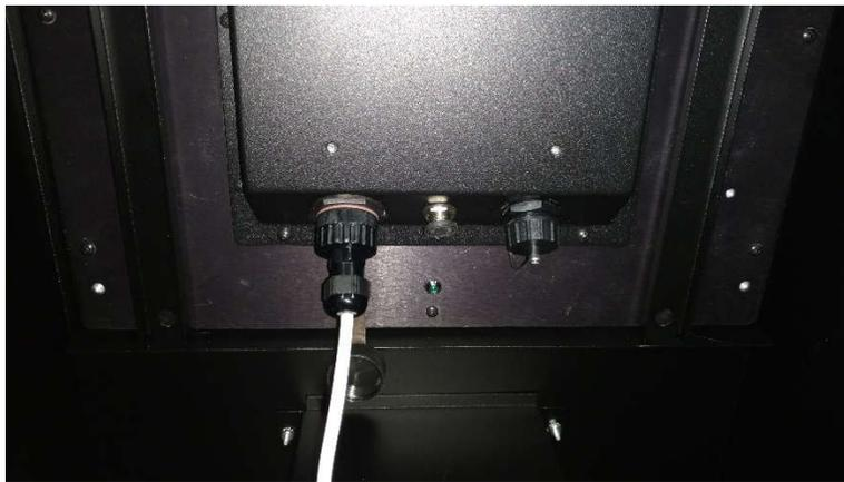
**Figure 19 - Watertight Connection**
