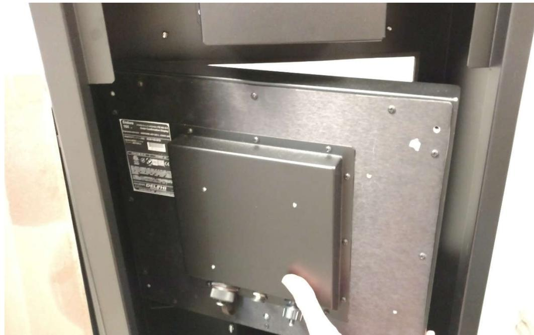
Figure 15 - Insert Endura 15X at an angle
