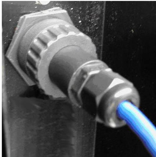
**Figure 11 - Properly Connected Cat5 cable**
