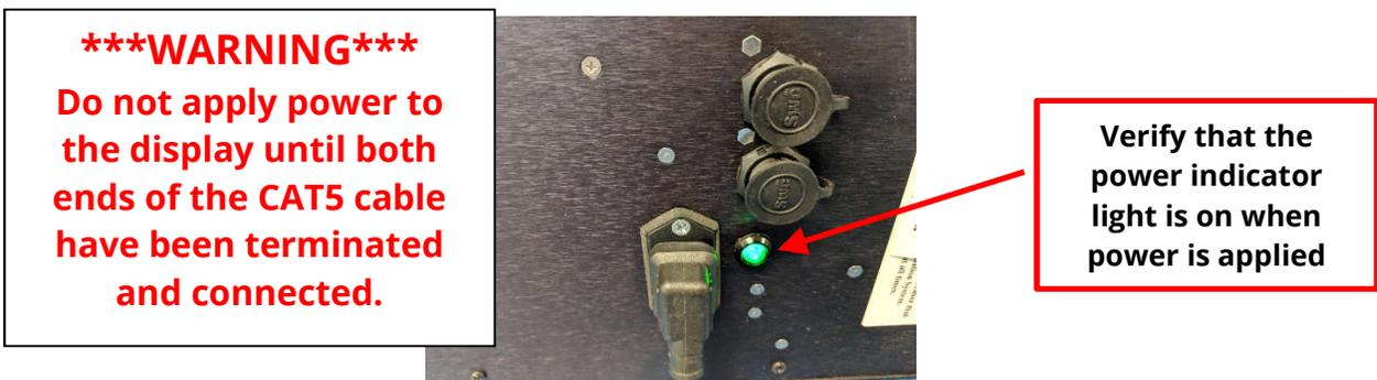
Figure 14 - Display Power Connection
