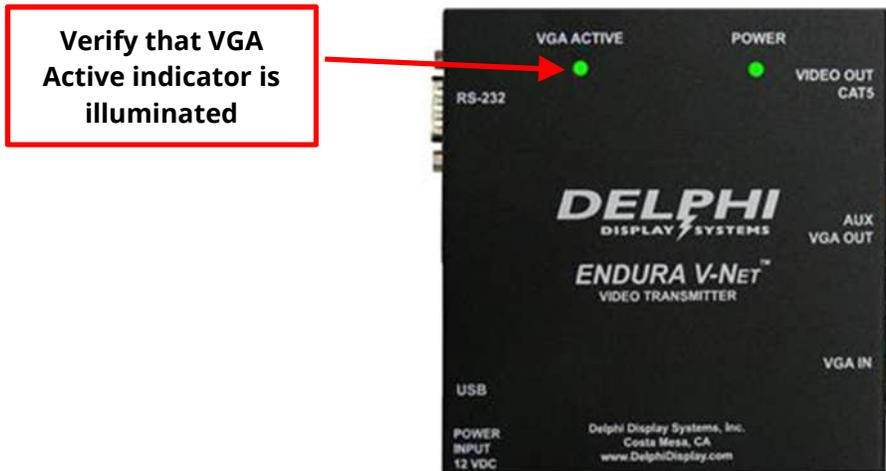
If there is no active VGA video signal on the VGA IN video input, the VGA ACTIVE light will not be illuminated. In this case, check the video connection to the video server. An external VGA monitor can be connected to the AUX VGA OUT connector to verify video is present on the VGA IN connector.
